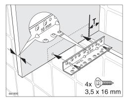
■ Screw the brackets onto the right and left inside walls of the housing unit as shown. The back edge of the brackets should align with the vertical line drawn up from the front of the spacer strip, and the lower edge aligned with the lower edge of the housing unit side wall.
